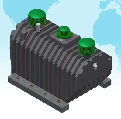
When the J-500-800 PLT is to be installed in areas where high water tables are common, additional anti-buoyancy measures should be installed. Jet recommends using concrete anchors placed beside the tank in the excavation and secured to the tank with properly rated corrosion resistant straps. Straps may be routed through the lifting lugs on the tank to ensure they will not shift during installation and backfilling.
