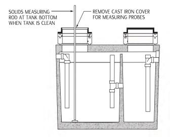
Obtain the FOG and/or solid levels using a "Sludge Judge" or a simple rod with a flat bottom piece to feel the mass levels within the recognized areas of separation, floatation and settling.
